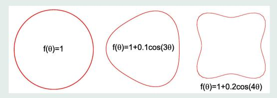
Figure 2.1. The Frank diagram of anisotropy.
