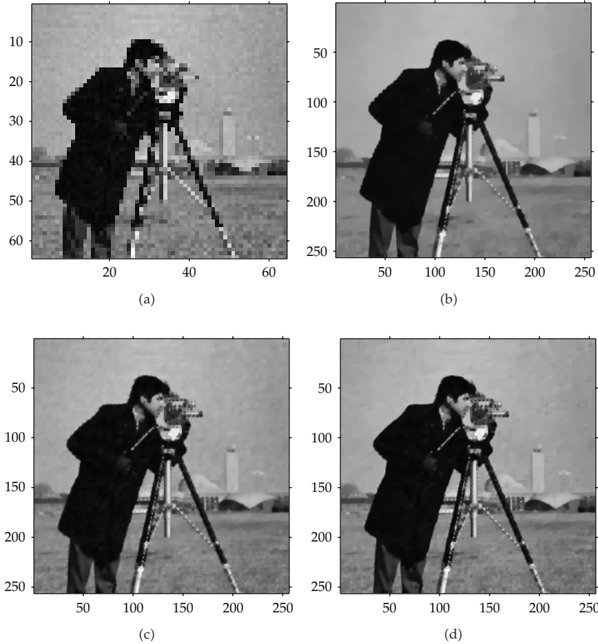
Figure 5: Results of different resolution enhancement methods applied to “Cameraman” image degraded by Gaussian blur with support size 3 \times 3 , standard deviation 0.5, and Gaussian noise with variance 20. (a) One LR image; reconstructed image (b) using LDFP method, (c) using AMM method, and (d) using the proposed method ( \mu = 130 ).
