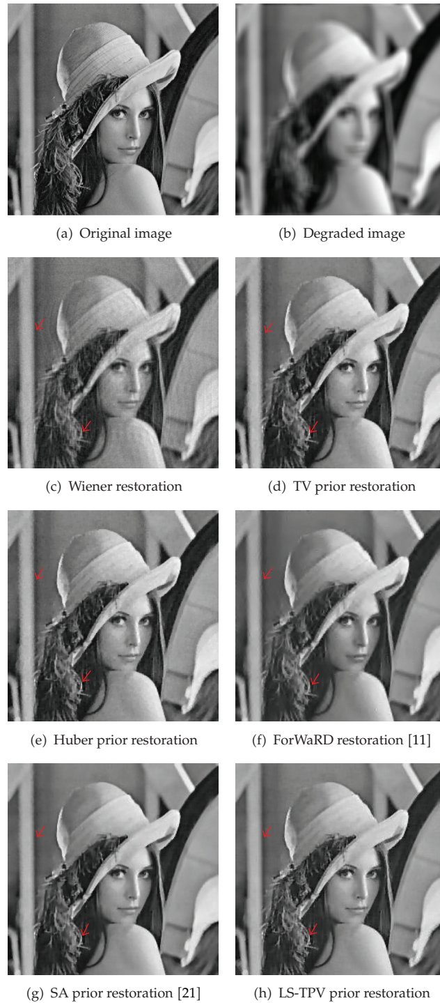
Figure 1: (a) Original “Lena” image. (b) Degraded “Lena” image (SNR = 6.65) with 9 \times 9 uniform blur and additive white Gaussian noise (variance = 0.1663). (c) Wiener deconvolution. (d) TV prior Bayesian restoration. (e) Nonquadratic Huber prior Bayesian restoration. (f) The ForWaRD restoration in [11]. (g) The SA prior Bayesian restoration proposed in [21]. (h) The proposed LS-TPV prior Bayesian restoration (The left arrows: block-suppressing illustration, the right arrows: edge-preserving illustration).
