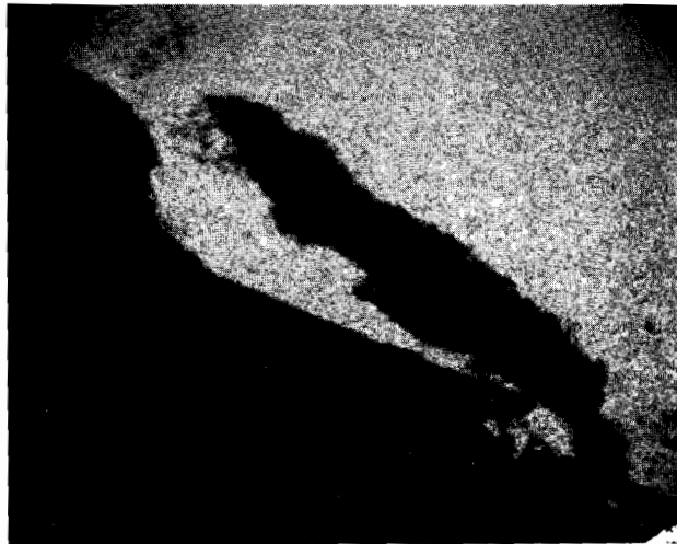
Fig. 1d. S-distribution picture. The area in which the eutectic form of the Ni-rich phase occurs shows also a gradual depletion in sulphur.
