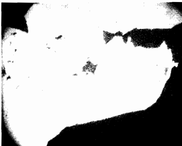
Fig. 3b. Cr-distribution picture. Some "holes" are suspicious, and were shown in the sulphur picture to be troilite inclusions.
