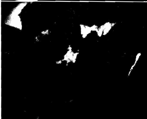
Fig. 3c. Sulphur distribution picture. It can be seen very clearly that there are troilite inclusions within the chromite inclusion (which is itself placed at the border of a large troilite nodule).
