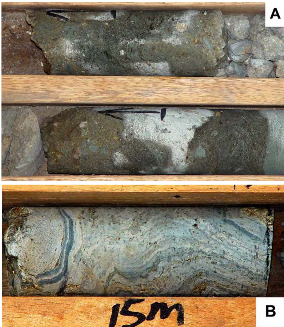
Fig. 5. The macroscopic appearance of suevite in Bosumtwi drill cores outside the crater rim. Note (a) the vesicular nature of the impact glass in the suevite from drill hole BH1 (depth is 10.2 m for the top part and 11.3 m for the bottom part), and (b) melt glass with flow structure in a suevite from drill hole BH3 (depth 15 m). The core diameter is 5 cm.
