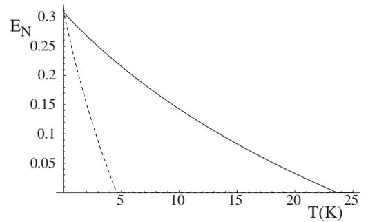
FIG. 2. Plot of the logarithmic negativity  $E_{\mathcal{N}}$  versus the mirror temperature. The solid line refers to a mass  $m = 5$  ng, detuning  $\Delta = w_m$ , and finesse  $\mathcal{F} = 1.07 \times 10^4$ ; the dashed line refers to a mass  $m = 50$  ng,  $\Delta = w_m/2$ , and finesse  $\mathcal{F} = 3.4 \times 10^4$ . The other parameters are those of Fig. 1.
