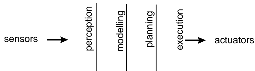
Figure 6: Traditional decomposition of robot control. Adapted from Brooks (1986).
