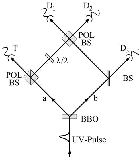
FIG. 1. Schematic drawing of the experimental setup for the demonstration of the Greenberger-Horne-Zeilinger entanglement for spatially separated photons. Conditioned on the registration of one photon at the trigger detector T, the three photons registered at  $D_1$ ,  $D_2$ , and  $D_3$  exhibit the desired GHZ correlations.
