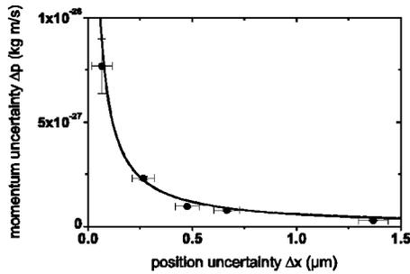
FIG. 4. Experimental verification of the Heisenberg uncertainty relation for  $C_{70}$ . The momentum uncertainty values  $\Delta p$  are derived from the far-field molecular-beam widths  $W_{\text{exp}}$  as described in the text. The position uncertainty  $\Delta x$  is given by the width of the second slit. The continuous line represents the expectation of a wave model for a monochromatic plane wave passing a slit.
