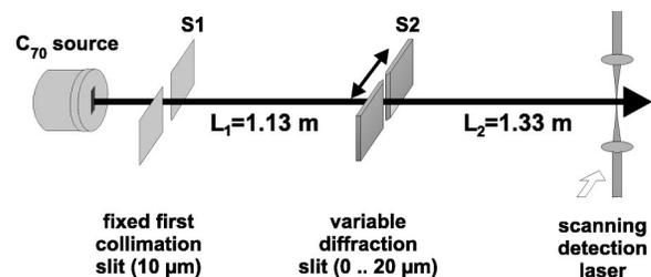
FIG. 1. Setup of the experiment. A thermal  $C_{70}$  beam is produced by sublimation of fullerene powder at 900 K. The beam is narrowed by  $S_1$  and diffracted by  $S_2$ .  $S_1$  is fixed at  $10 \mu\text{m}$ . The width of slit  $S_2$  is varied with  $\pm 30$  nm accuracy for  $\Delta x < 1 \mu\text{m}$ .
