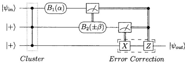
Fig. 1. Circuit diagram showing the principle idea of error correction via feed forward for one-way quantum computing.
